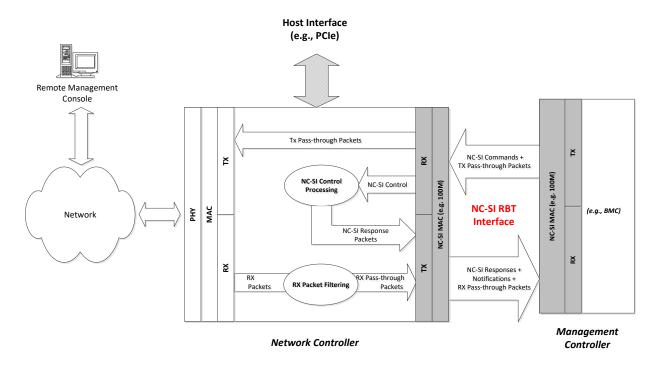
Figure 1 - NC-SI over RBT traffic flow diagram
