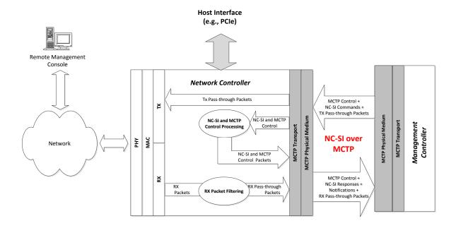
Figure 2 - NC-SI over MCTP traffic flow diagram
