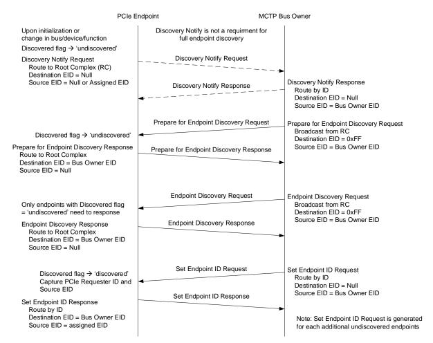
Figure 2 - Flow of operations for full MCTP discovery over PCle
