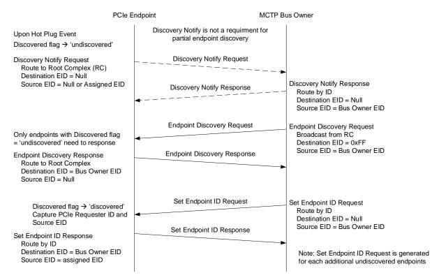
Figure 3 - Flow of operations for partial Endpoint Discovery
